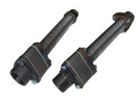
The ESKAY Tri-Valve Assemblies offer a flexible connection with a non-return valve between the pipework and the pump unit. The Assemblies come in various configurations both with and without the non-return Triangle Valve. The non-return Triangle valve can have either a nitrile or viton poppet.
