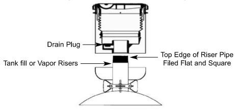
1. Before installing the A1004EVR spill containment, the top edge of the riser pipe must be filed flat and square to insure a proper sealing surface between the riser pipe and base of the 1004EVR spill containment.
